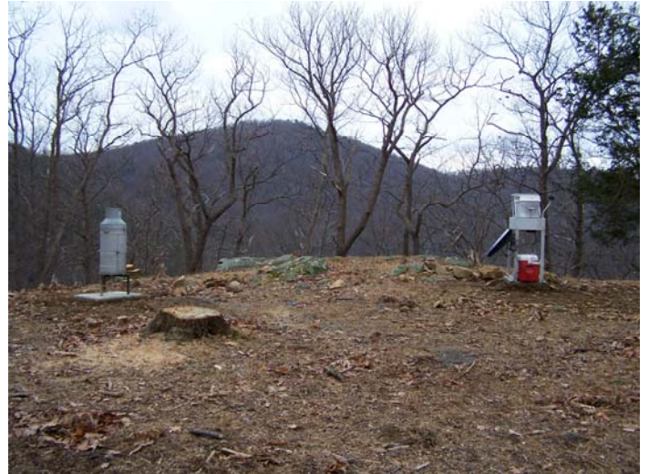
Preparing the new NADP site (left) and the monitoring station, with rain gauge on left and precipitation collector on right (right).
